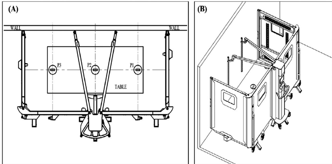
**Fig 1.** (A) Top view and (B) isometric view of the test equipment in rectangular configuration surrounding a table with triplicate test samples equally spaced in the center of the 195 × 140 × 274 cm FMUV target zone.
